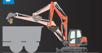
B High dumping reach
